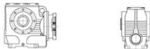
SA(S, SF, SAF, SAZ) ...Y... Customers provide the motor by themselves need connected flange.
